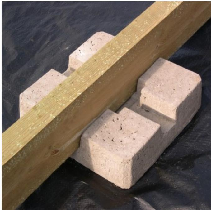
Moulded into the top of each deck pier are slots and a square recess. The slots on a concrete Deck Pier hold 47mm joists and the hole is for a 100 x 100mm post - necessary when building on uneven terrain or creating different deck levels.
