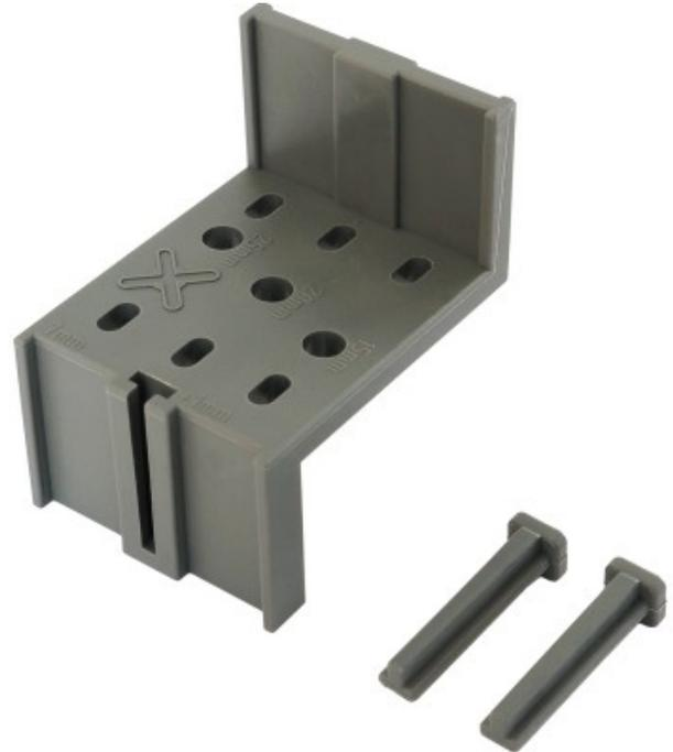
The Decking Installation Aid is a clever device designed to help create a consistent gap between deck boards and to help quickly position screws in the exact location on the deck board. This not only speeds up the installation process, but also helps make the finished deck neater and more visually appealing by helping to ensure that gaps between boards are equal and the screws are in the exact same position on the deck board throughout.
